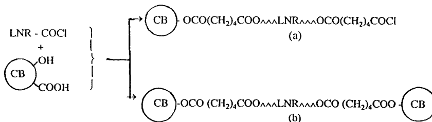
SCHEME 1. Preparation of LNR-grafted carbon black.
